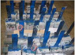
**Figure 3. Anchorage Test Specimens**
