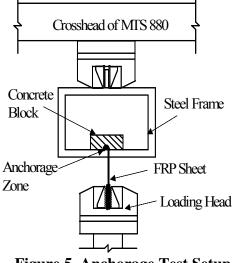
Figure 5. Anchorage Test Setup
