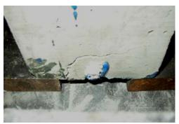
Figure 11. Anchorage Failure Mode
