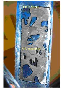
Figure 7. Failure Mode between FRP Sheet and VE Layer
